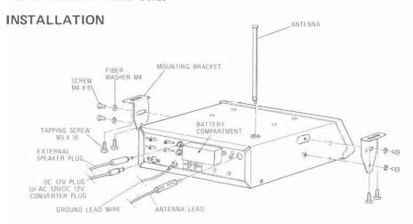
NOTES: BATTERY INSTALLATION: Before turning your SX-200 on make certain that you install the two SIZE AA BATTERIES supplied in the battery housing on the rear panel being careful to put them in with the correct polarity (Polarity is marked on base of plastic holder.) The batteries are used for memory backup.
